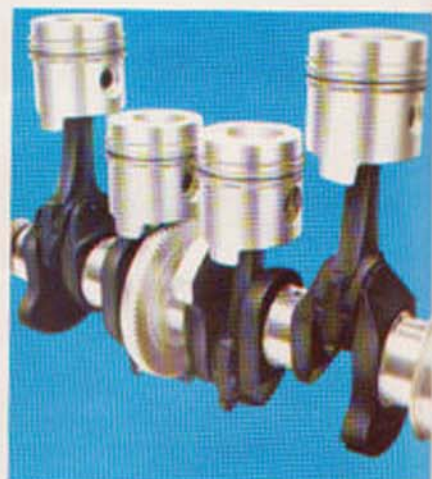
Five-bearing crankshaft offers strength and rigidity for smooth operation, durability.
