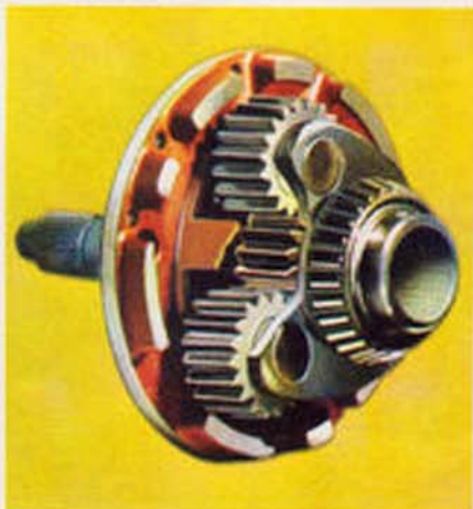
Double-reduction rear axle incorporates inboard planetary gears of high grade, heat-treated steel.
