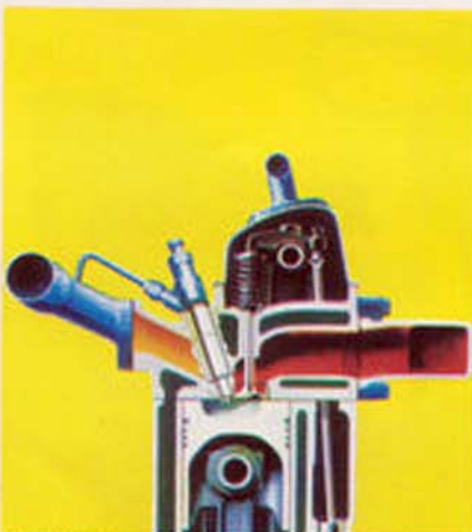
New diesel cylinder head with porting, combustion chamber and valve-shape revisions for cleaner, more economical running.
